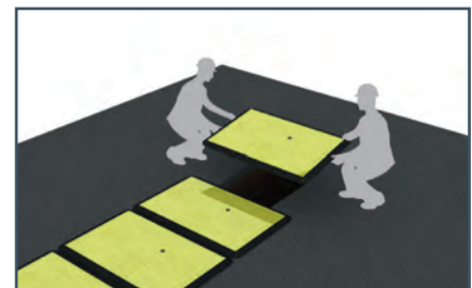
Repeat until the entire trench is covered.
